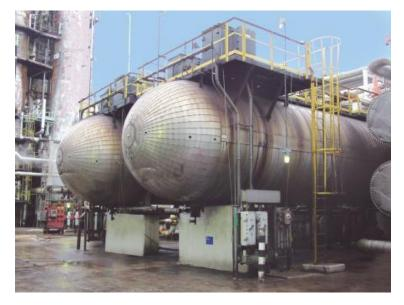
The salts contained in the brine left over from crude oil can cause serious corrosion and scaling problems and must be removed. Desalting removes salts and residual free water. Although the refinery is the most economical site for desalination, to protect pipeline, onsite desalting is required at the extraction site.
